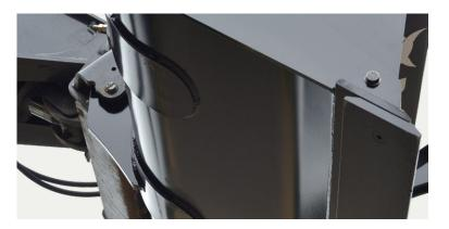
Bobcat buckets are shipped from the factory with pre drilled holes in the original front cutting edge.
